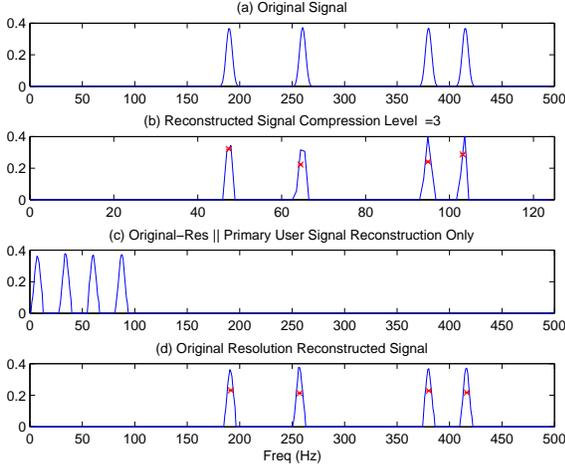
Fig. 3. MultiResolution Bayesian Compressive Sensing:  $K = 4$ ,  $M = 140$ ,  $N = 512$ ,  $\Gamma = 2 * 10^{-4}$ . (a) Original signal (b) Reconstructed lowest resolution signal (c) Original resolution reconstruction of only detected Primary User signal (d) Original resolution reconstructed signal
