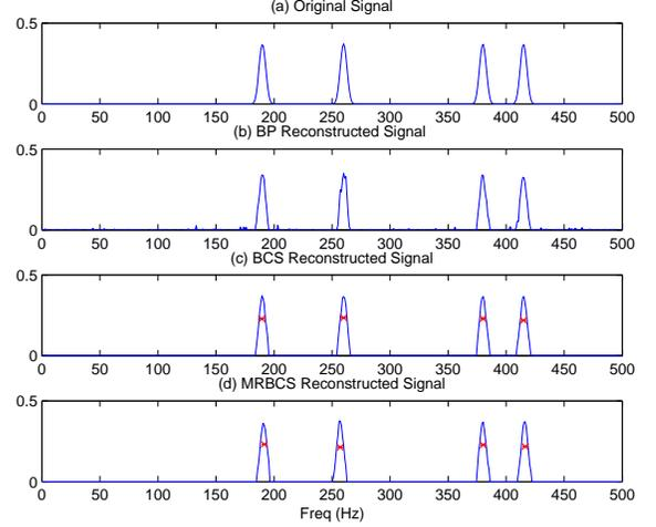
Fig. 4. Comparison of signal estimation using BP, BCS PU detection, and MRBCS PU detection for  $K = 6$ ,  $M = 160$ ,  $N = 512$ ,  $\Gamma = 2 * 10^{-4}$ . (a) Original signal, (b) Reconstruction with BP,  $t_{REC} = 1.3482$  secs (c) Reconstruction with BCS PU detection,  $t_{REC} = 0.3102$  secs (d) Reconstruction with MRBCS PU detection,  $t_{REC} = 0.0551$  secs
